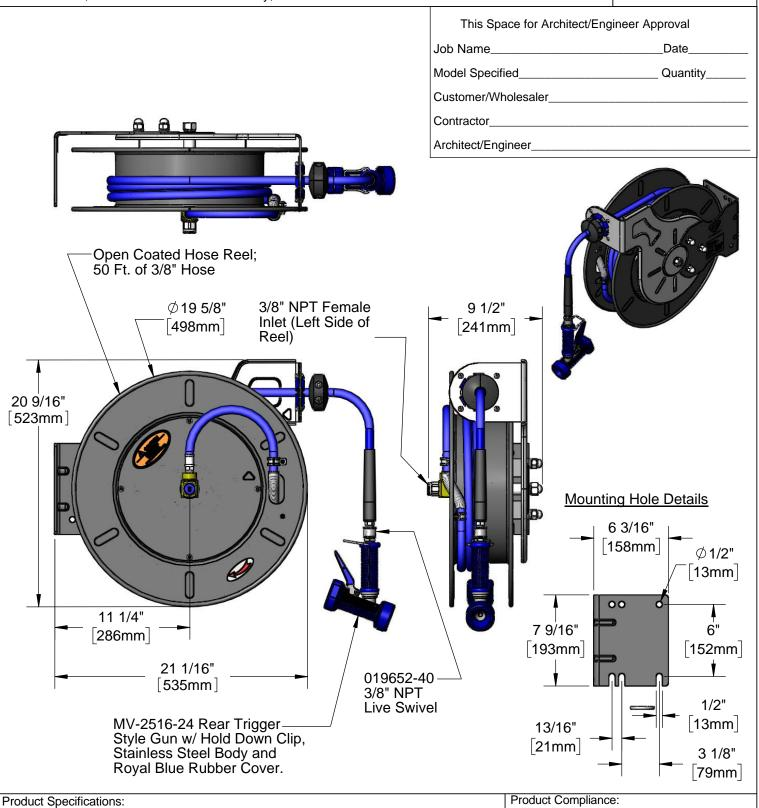
3/8" x 50 Ft. Open Coated Reel w/ Rear Trigger Spray Gun & Swivel,
